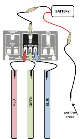
IMPORTANT TO KNOW: The electricity needs to travel a short distance to get to the red connection, but a much longer distance to get to the green connection. This means there is more electrical current at the red connection than at the green connection. The red light of the LED will be brighter than the green light.
